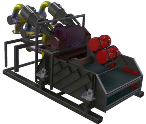
Removable Equipment Skid for De-Sanding Unit for Non Routine Maintenance
